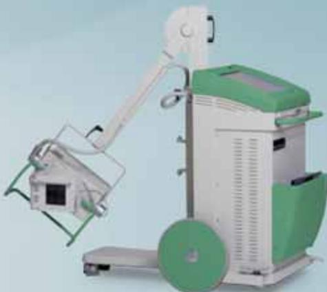
*Mobile Unit equipped with digital images acquisition system in radiography mode with detector at solid status.*
